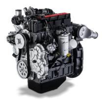
In terms of sustainability, the F28 engine meets **Stage V and Tier 4 Final emission standards**, featuring **FPT Industrial's extremely compact after-treatment system**. This solution uses a Diesel Oxidation Catalyst (DOC) with a Diesel Particulate Filter (DPF), allowing the same engine to **meet both European and North American emissions regulations while guaranteeing consistently high-power delivery**.
