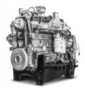
Engine power has been increased to 250 kW, a 9% increase in maximum power and torque compared to the previous model, and enabling the use of larger implements or faster working speeds for increased productivity. Maximum cylinder pressure has been increased to 180 bar (+20 bar) for higher combustion efficiency, while the improved design of the pistons,
